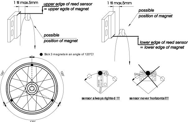
For fixation on the rear wheel the cable can be extended. A shielding in the range of ignition is recommended.
